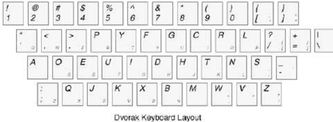
Figure 2: The Dvorak layout. The small letters in the corners represent the QWERTY layout.
